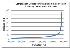
\*Specimen Area: 1inch<sup>2</sup> Rate of strain= 1.0mm/min
