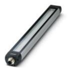
LED machine light, 24 V DC, emission angle 85 °/95 °, color temperature 5000 K, length 365 mm, diameter 40 mm, M12 connector, Light housing: Anodized aluminum, Pane: Single-pane safety glass (ESG, thermally toughened float glass), pivoting, resistant to coolants and lubricants
