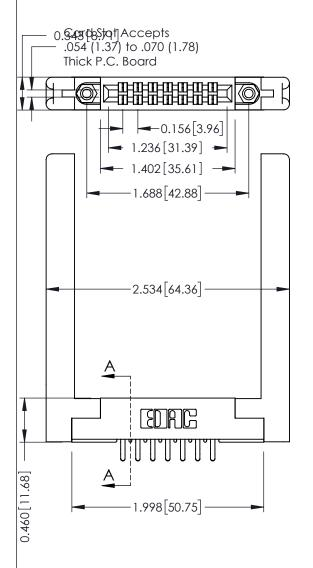
0.295[7.49] Card Slot ECTION 0.090[2.29] Point of Contact 305 ENG MASTER 305 / 315 / 355 Card Edge Connector J.LEE DATE: SEPT. 21/09 Part Number: 315-014-556-258
