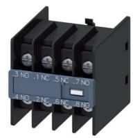
Auxiliary switch 11 U, on the front, 2 NO + 2 NC Current path 1 NO, 1 NC, 1 NC, 1 NO for 3RH and 3RT Ring cable lug connection .3/.4, .1/.2, .5/.6, .7/.8
