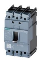
circuit breaker 3VA5 UL frame 125 breaking capacity class M 35kA @ 480 V 3-pole, line protection TM210, FTFM, In=20A overload protection Ir=20A fixed short-circuit protection Ii=15 x In UL489 SB (naval), 50 deg. cel. cable connection on both sides
