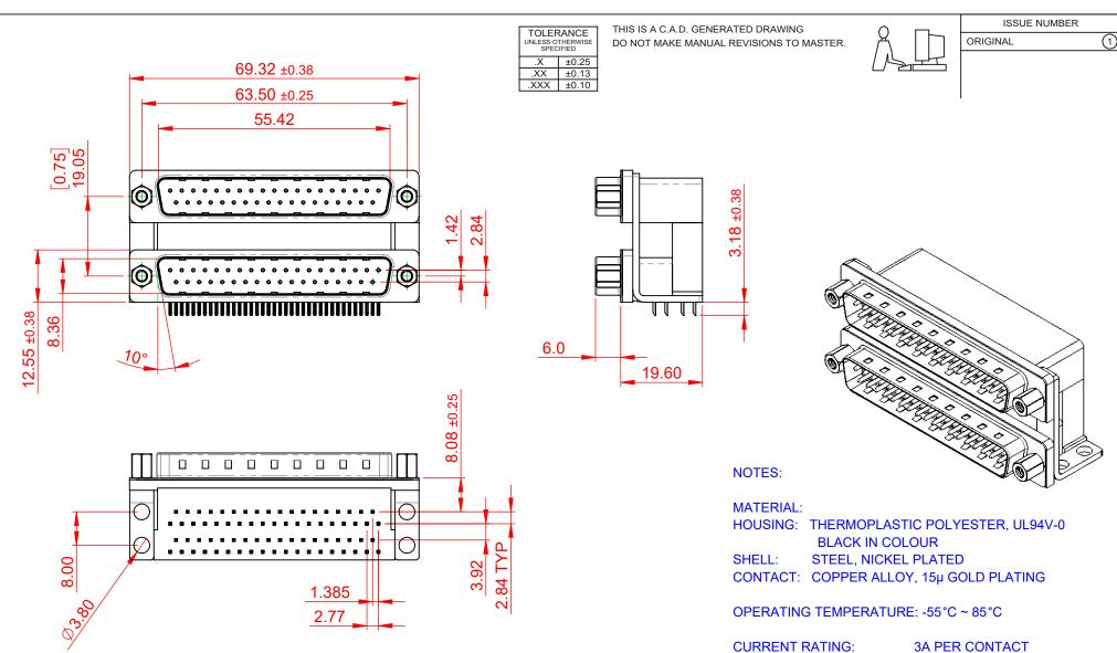
CURRENT RATING: 3A PER CONTA CONTACT RESISTANCE: 25mΩ MAX. INSULATOR RESISTANCE: 5000MΩ min. DIELECTRIC WITHSTANDING VOLTAGE: 1000V AC rms
