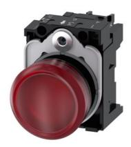
Indicator lights, 22 mm, round, plastic, red, lens, smooth, with holder, LED module, with integrated LED 24 V AC/DC, screw terminal, with laser labeling, inscription or symbol Customer-specific selection with SIRIUS ACT configurator (CIN)
