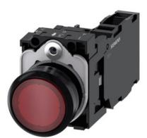
Illuminated pushbutton, 22 mm, round, plastic, red, pushbutton, flat, momentary contact type, with holder, 1 NO+1 NC, LED module with integrated LED 110 V AC, screw terminal, with laser labeling, upper case
