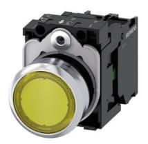
Illuminated pushbutton, 22 mm, round, metal, shiny, yellow, pushbutton, flat, momentary contact type, with holder, 1NO, LED module with integrated LED 24 V AC/DC, screw terminal, with laser labeling, upper case and lower case, always upper case at beginning of line
