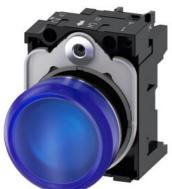
Indicator lights, 22 mm, round, Metal, shiny, blue, lens, smooth, with holder, LED module with integrated LED 230 V AC, screw terminal, with laser labeling, symbol number according to, ISO 7000 or IEC 60417
