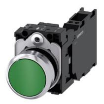
Pushbutton, 22 mm, round, metal, shiny, green, pushbutton, flat, momentary contact type, 1 NO+1 NC, spring-type terminal, with laser labeling, inscription or symbol Customer-specific selection with SIRIUS ACT configurator (CIN)
