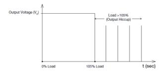
Additionally, if the  $I_0$  is <250% but >110% for a prolong period of time (depending on the load), the Over Temperature Protection (OTP) will be activated due to high temperature on critical components. The power supply will then go into hiccup mode until the fault is removed; and, the input voltage is removed, then reapplied.
