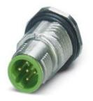
Sensor/actuator flush-type plug, with green contact carrier, 5-pos., M12 SPEEDCON, shielded, B-coded, rear/ screw mounting with M16 thread, with straight solder connection
