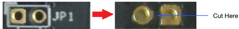
Figure 6. Top and Bottom View of Shorted Jumper. The Bottom View Shows the Trace Location to Cut for Current Measurement
